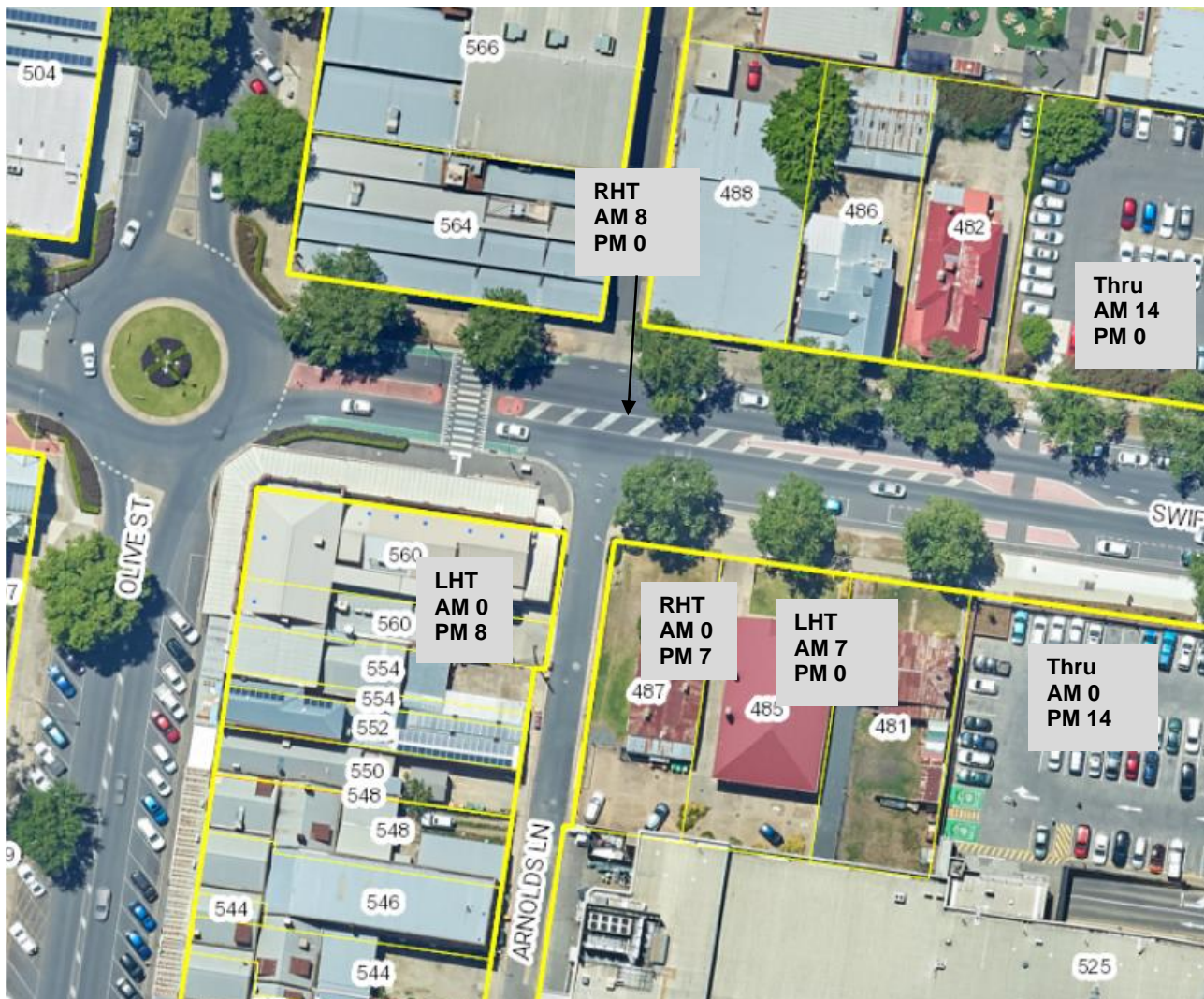
Figure 2: Additional AM and PM peak hour turning movements at intersection Swift Street and Arnolds Lane
