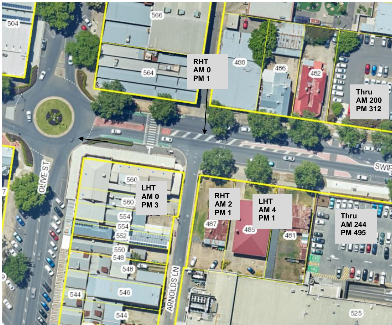
Figure 1: Summary of existing AM and PM peak hour turning movements at intersection of Swift Street and Arnolds Lane
